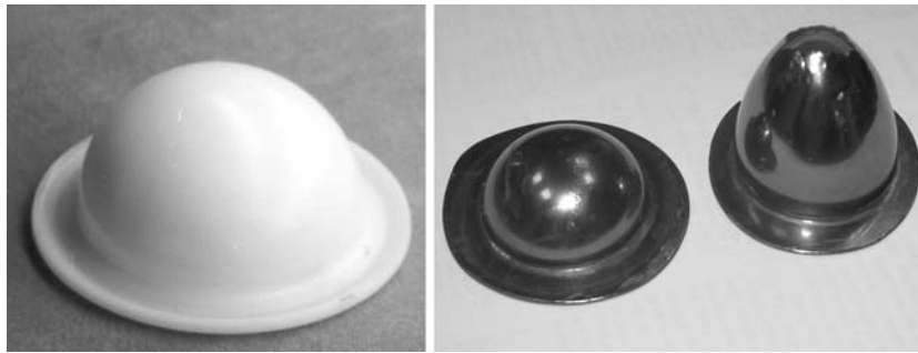
Fig. 40 First bubbles superplastically formed from ceramic sheet (1992) and from bulk glass Zr.Ti.Ni.Cu.Be alloy (2006)
