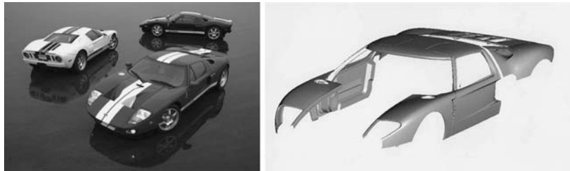
Fig. 31 Forty years after its debut, the modern Ford GT supercar is clad with 10 superplastically formed, SP5083 alloy, body panels
