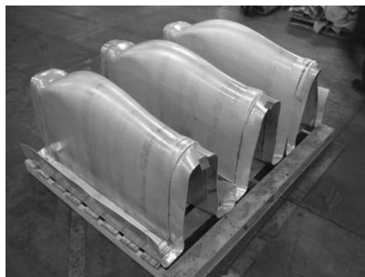
Fig. 20 More uniform thickness distribution resulting from non-planar clampline forming
