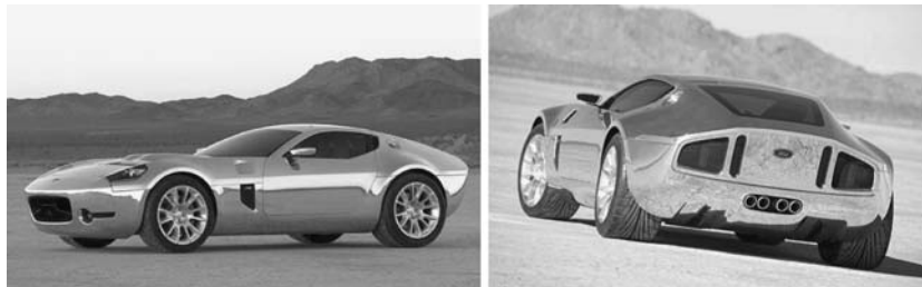
Fig. 32 The complete body of this 2005 showcar was SPF'ed in SP5083 alloy using low cost, 'cast to size' aluminum tooling
