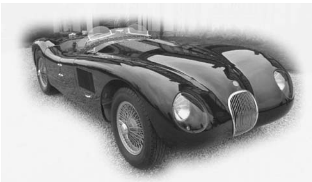
Fig. 33 A fusion of old and new, superplastic forming technology makes this 2006 limited series reproduction of the 1954 classic Jaguar C-Type a practical reality
