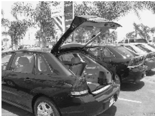
Fig. 22 GM Malibu Maxx with QPF liftgate formed from SP5083 alloy
