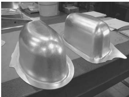
Fig. 23 Male formed C17 hydraulic covers made from SP2004 and heat treated to the T-6 condition
