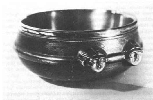
Fig. 13 Russian decorative sugar basin—one of thousands produced from Bochvor's Zn Al Alloy
