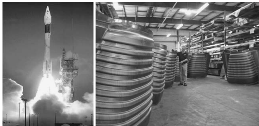
Fig. 29 Structurally critical launch vehicle components formed from SP7475 alloy
